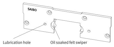
The plastic lubrication covers contain oil soaked felt wiper which can be re-lubricated via lubrication holes shown above.
